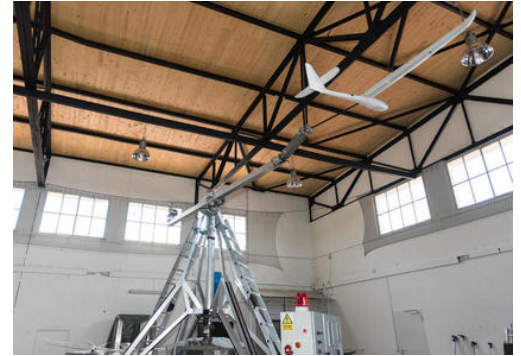
Experimental trial of a half-wing kite in rotational-start, controlled with nonlinear model predictive control.
