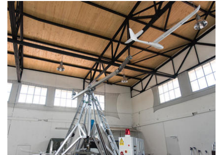
Experimental trial of a half-wing kite in rotational-start, controlled with non-linear model predictive control.
